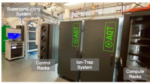
Fig. 1: A view into the Quantum Integration Centre (QIC) at LRZ/Munich showing a superconducting system (left), an ion-trap system (middle) and HPC racks covering the classic compute. The result is a strongly disaggregated infrastructure combining classical HPC clusters with large-scale accelerator
